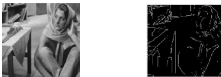
Fig.2. Image processing (a) After Averaging Template (b) After Averaging and Edge Detection
